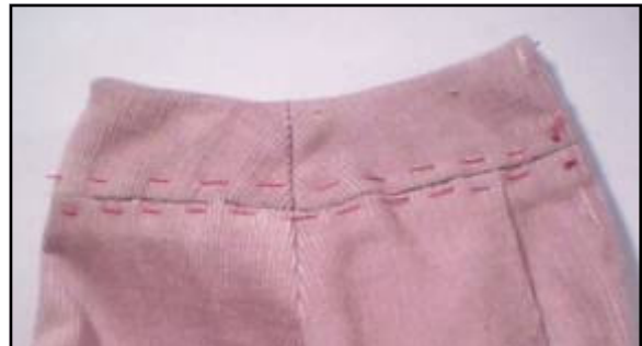
“Stitch in the Ditch” from the outside. (Black thread illustrates how the stitching runs inside the seam that joins the waistband to the body of the skirt.)
