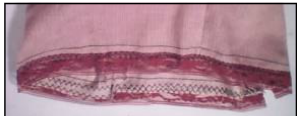
Hem tape zigzagged to the bottom of the skirt. The black stay stitching above the hem tape is where the hem will fold over.
